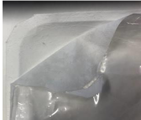
Separation plastic laminated film from cardboard (ex. 1)
