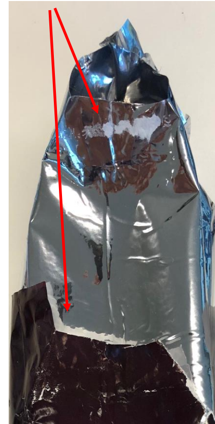
4. Little adhesive used → paper and aluminium layer can be separated easily
