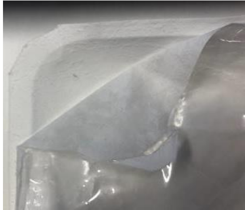
2. Separation plastic laminated film from cardboard (ex. 1)
